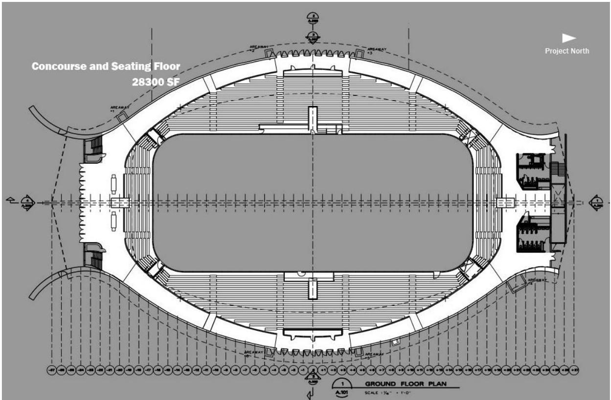
Figure 14 | Ground Floor Plan – Concourse and Seating Floor
